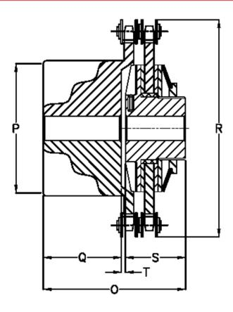
Max angular displacement = 30 S = 65Max parallel displacement = 0.35 T = 3.0Max torque Nm = 190Number of springs = 1 0 = 110.0 Ρ = 90 Q = 42.0R = 138.0
